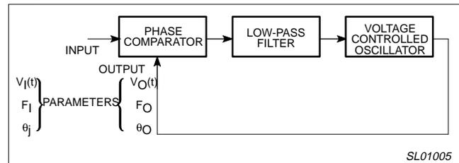
Figure 1. Block Diagram of a Phase-Locked Loop
